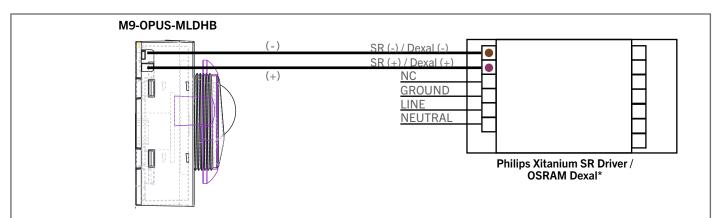
\*When wiring the M9-OPUS-MLDHB to a DALI driver other than the Philips Xitanium SR Driver or Osram Dexal, please refer to the connections labeled on the device to find the (-) and (+) receptacles.
