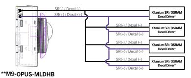
\*\*Respect Xitanium SR / OSRAM Dexal bus polarity when more than one Xitanium SR / Dexal LED is connected in parallel.
