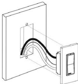
NOTE: Dress wires with a bend as shown in diagram in order to relieve stress when mounting ILS2
