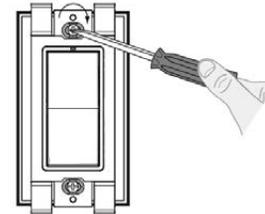
Tighten mounting screws to secure the device to the wall box.
