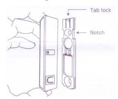
b. Position the mounting bracket and mark the two mounting screw drill points.
