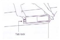
f. Slide the sensor on the bracket until it snaps into place on the tab lock.
