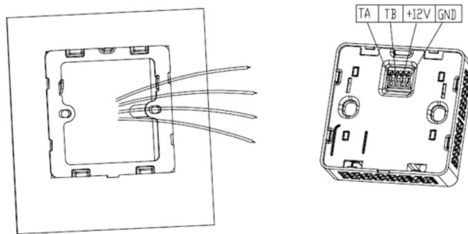
Step 3: Match the two holes in the controller with the hooks in the wall mount bracket and slide the controller down to ensure that the controller is tightly locked with the bracket.
