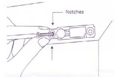
d. Install the second screw, and then hand-tighten the first screw.
