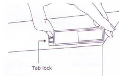
f. Slide the sensor on the bracket until it snaps into place on the tab lock.
