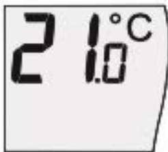
The setpoint can only be changed in comfort mode. Only the setpoint for comfort mode can be changed.
