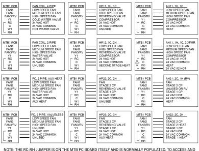
NOTE: THE RC-RH JUMPER IS ON THE MTB PC BOARD ITSELF AND IS NORMALLY POPULATED. TO ACCESS AND CUT THAT JUMPER, THE BOARD MUST BE REMOVED FROM THE CASE. USE FLUSH CUTTING PLIERS.
