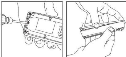
3. Remove the installed lens by gently squeezing it to ease one side out of its groove, and then the other.
