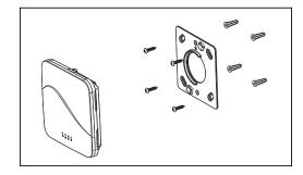
• Attach device to backplate by aligning tabs and twisting / locking into place (see below)
