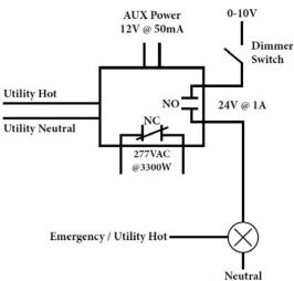
This is the same case as above, however, only a low voltage dimmer switch is controlling the fixture. When our 'ALCR' senses the loss of normal power, the 24V relay opens and breaks the circuit, forcing the light fixture to go to a full on state.
