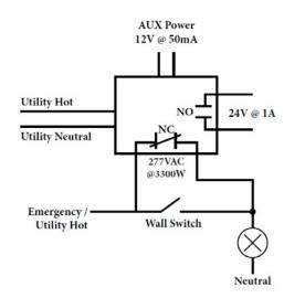
Normal/emergency lights are fed via a normal/emergency breaker panel and a wall switch, wall box dimmer, or other wall-box-mounted control device. When normal power fails, an upstream UL 1008 emergency transfer switch automatically transfers the feeder of the breaker panel to an emergency power source. At the same time, our 'ALCR' senses the loss of normal power and bypasses the switch or dimmer, forcing the load on, no matter what the position of the switch or dimmer.
