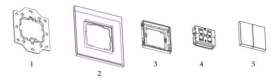
**WE SUGGEST MOUNTING ON A SOLID SURFACE:** Depending on the ground (brick plaster, glass...) the base plate can be glued or screwed. In any case, the ground must be smooth. Unevenness can lead to malfunctions! Watch that no dust is getting inside the housing.
